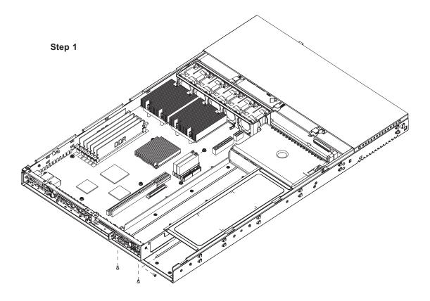
Figure 6-6. Reconfiguring the Power Supply
